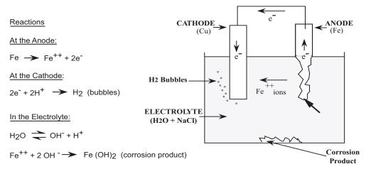
Figure 1A Typical Galvanic Cell
