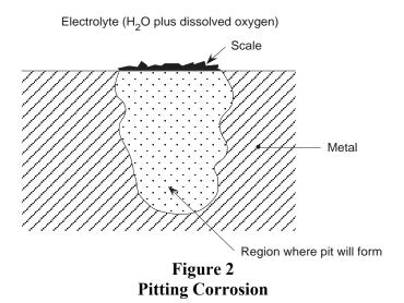
Pitting and crevice corrosion are minimized by chemical control, proper drainage of vessels during shutdown, removal of suspended solids by filtration, removal of corrosion products by ion exchange, and removal of scale, crud and bacterial deposits.
